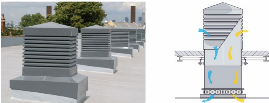
Fig. 4.2.1. Torre de viento “Windcatcher Classic System” (Monodraught)
