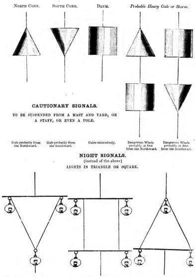
Four lanterns and two yards, each not less than four feet long, will be sufficient — as only one signal will be used at night. These signals may be made with any lanterns, showing either white, or any colour, but dike. Red u most clightle. Lamps are preferable to candles. The halvards should be good rope, and protected from chafing. The lanterns should hang all least three feet apart.
